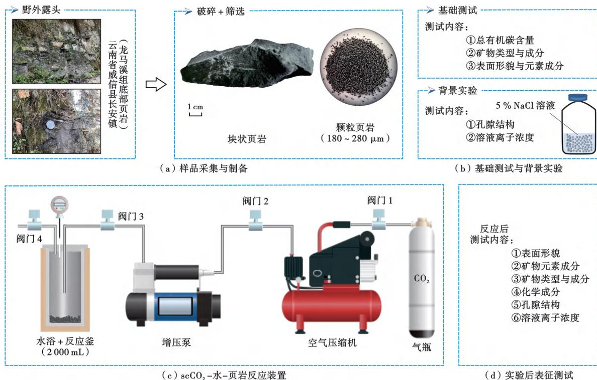
图2  $\text{scCO}_2$ -水-页岩反应的实验流程Fig. 2 Experimental flow of  $\text{scCO}_2$ -water-shale reaction
